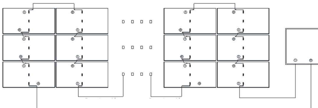
**Fig. 9-4 Horizontal installation of long cable modules**
